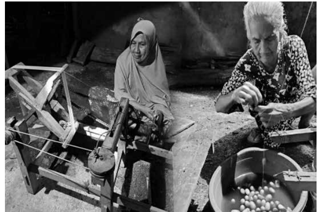
Figure 4. Spinning Silk from Cocoons using Traditional Hand-Spinning Tools
